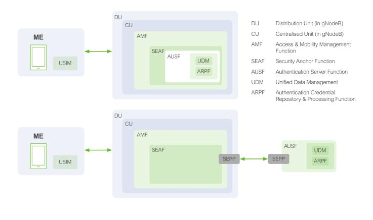
Figure 3. (a) 5G Trust model and (b) 5G Trust model for roaming scenario
