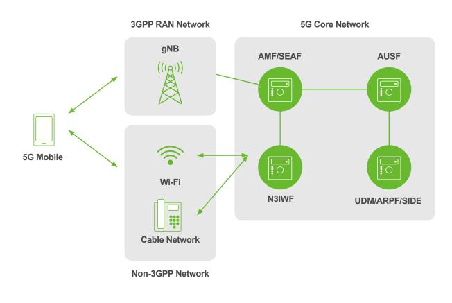
Figure 5. Two ways of accessing a 5G network. AMF (Access and Mobility Management Function), SEAF (Security Anchor Function), AUSF (Authentication Server Function), UDM (Unified Data Management), ARPF (Authentication Credential Repository and Processing Function), SIDF (Subscription Identifier Deconcealing Function), N3IWF (Non-3GPP Interworking Function).
