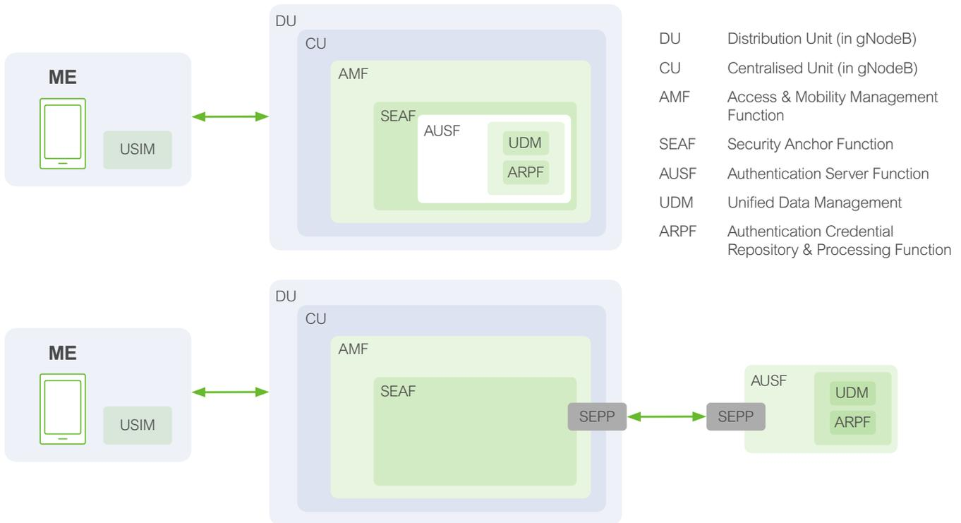
Figure 3. (a) 5G Trust model and (b) 5G Trust model for roaming scenario
