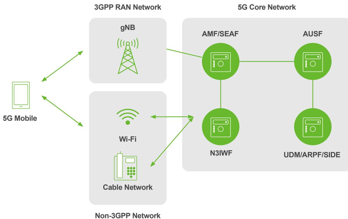
Figure 5. Two ways of accessing a 5G network. AMF (Access and Mobility Management Function), SEAF (Security Anchor Function), AUSF (Authentication Server Function), UDM (Unified Data Management), ARPF (Authentication Credential Repository and Processing Function), SIDF (Subscription Identifier De-concealing Function), N3IWF (Non-3GPP Interworking Function).
