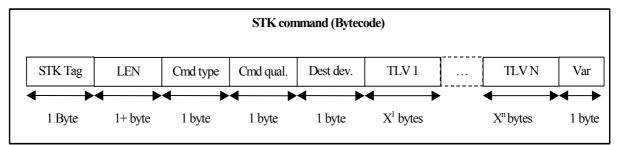
The structure of the byte code value field representing a simple STK command is the following:
