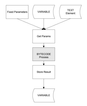
Each byte code takes parameters for input (fixed, variables or text elements), processes them and provides an output that is stored in an output variable. Some byte codes may have no output (as switch case for example).
