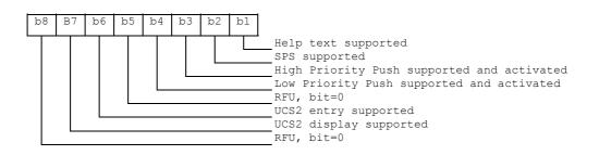
During each initialisation procedure the terminal profile is evaluated and a logical 'and' operation is being executed between the browser and the mobile facility indication flags, e.g. an indication of an UCS2 entry support means, that both the browser and the mobile phone support this facility.
