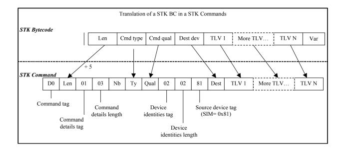
All TLV parameters of this byte code are parsed for variable substitution as explained in next paragraph. Processing of output values is defined just after.
